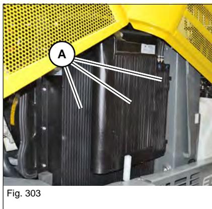
Radiators **A** are located on the right in the engine compartment.
