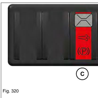
**C:** Parking brake switch for standstill regeneration ET90 DPF
