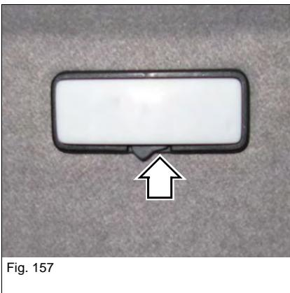
The mechanical switch above the left B-pillar must be in the position on the right so that the interior light can be switched on and off with the help of the switch panel.
