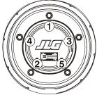
Figure 33. Wheel Lug Nut Tightening Sequence
