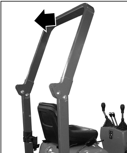
Fig. 83: Lowering the rollbar
