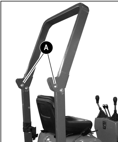
Fig. 82: Lowering the rollbar
