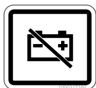
Fig. 21: Battery master switch
