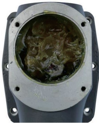
Figure 3 new grease example (before any single use)
