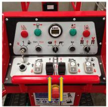
High speed will activate automatically after approximately 5 seconds when maintaining full speed on the toggles.
