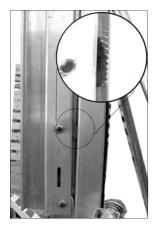
When the brake is engaged, it will be possible to see the Brake Cam acting on the adjacent mast section.
