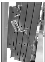
The winch handles have been placed in the stored position.
