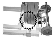
Pull the tool down and the brake will release.
